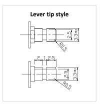
**DIMENSION** Unit: mm Circuit diagram Viewed from the direction A **Dimensions** No P.C. board mounting hole dimensions (viewed from the direction A) TOTAL TRAVEL TRAVEL MOUNTING FACE (SELF LOCK)◀ 8-01.3.905 HDL 1 2.5 P.C.BOARD MOUNTING FACE TERMINAL NO @ 6±0.2 TOTAL TRAVEL MOUNTING FACE (NON LOCK)**←** 2 8-01.3.49.05 HITL 0.5 P.C.BOARD MOUNTING FACE TERMINAL NO @ 2.5 2.5 6 ±0.2
